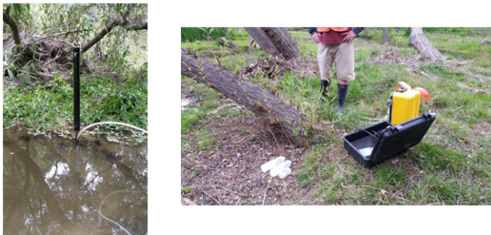
FIGURE 4. A peristaltic pump (right photo) is used to draw water samples into a mini-piezometer that is installed temporarily in both in-channel and off-channel hyporheic zone sites (left photo).
