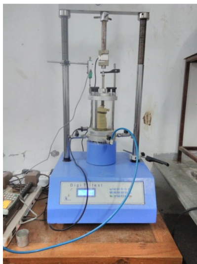
Figure 3. Triaxial Test on Reinforced Soil Specimen
