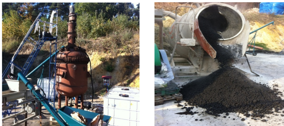
Figure. 2 The pilot plant for the production suspension and solid of mineral-organic fertilizers based on waste from poultry industry.
